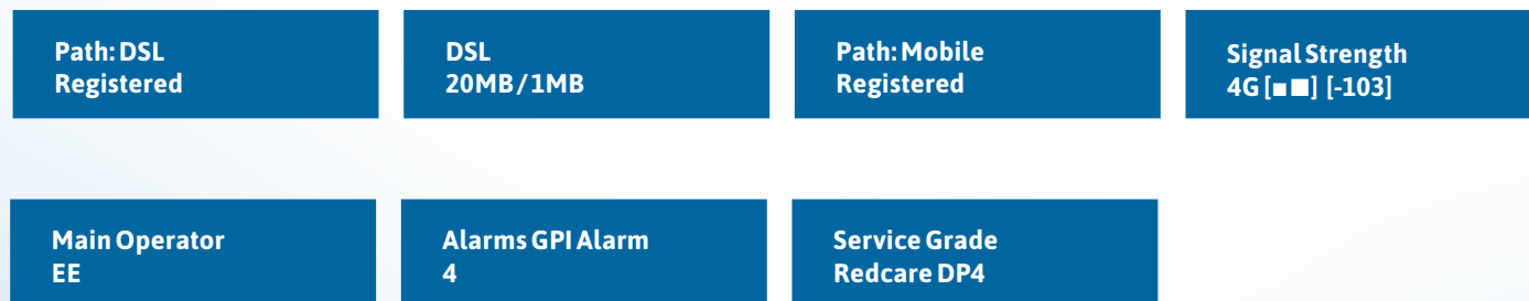
Figure 5 – Typical display cycling on a fully commissioned unit with a good signal strength and pin 4 in the alarm or open state
