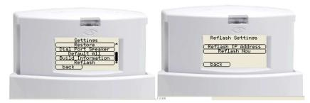
The reflash IP address is set by default to AddSecures's reflash server (195.59.117.164) and does not need to be changed unless another reflash server is to be used.
