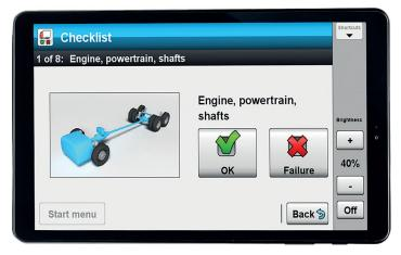
The driver goes through a checklist where the parts are highlighted.
