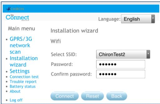
The IRIS Connect dialler will now show results of a Wi-Fi network scan for all current networks available. The networks found will be shown in the 'Select SSID' drop down box.
