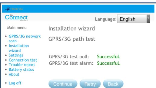
The IRIS Connect dialler will make a test poll and test alarm transmission over the GPRS/3G network.
