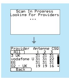
For a reliable 2/3/4G connection it is recommended that for the chosen network (SIM card) used there should be at least two base stations with signal strength (CSQ) of 10 or more.
