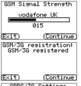
If you selected connection via GPRS/3G, the dialler will display the current operator / signal strength for the base station to which it is currently attached.
