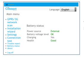
The IRIS Connect dialler allows installers to check the current battery status and will indicate any issues with the batteries.
