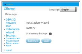
Note 1: If installing the IRIS Connect without batteries then please untick the 'Use battery backup' option.
