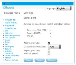
This allows you to setup the serial port for Texecom Premier Connections, Honeywell Galaxy RS485, or Normal modes. By default this is setup for Texecom emulation. For more information on the connection and setup please refer to the panel installation manual available from <u>http://www.chironsc.com/downloads\_security.html</u>.
