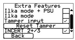
If the tamper physical condition has been restored before 'Reset Tamper' has been selected, the reset button will be removed and the tamper restore message will be sent to the monitoring centre. If not, the button will be removed and the tamper restore will be sent when the condition is restored.
