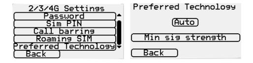
This setting allows the installer to select the preferred technology (Auto, 2G, 3G or 4G) used by the dialler for its cellular connection and the minimum signal strength required for the connection. If the signal strength is not at the required level (default is 10), the terminal will use
