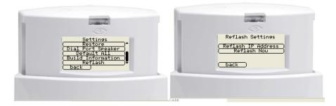
The reflash IP address is set by default to AddSecures's reflash server (195.59.117.164) and does not need to be changed unless another reflash server is to be used.
